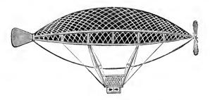
balloon. A small auxiliary balloon, situated inside the balloon, is inflated with air to compensate for the loss of gas.
